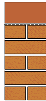
Brick on edge capping (not recommended - see notes)
