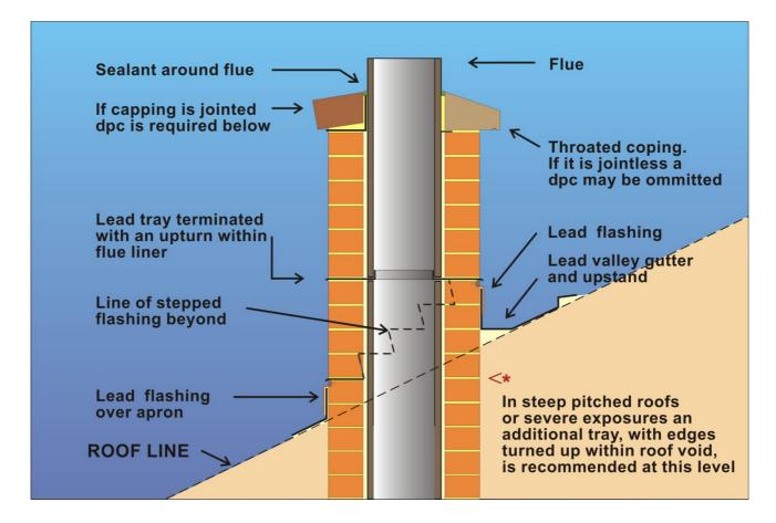
A brick-on-edge capping (or any mortar jointed capping or coping) will permit water to penetrate its joints and percolate down into the brickwork below. Therefore a flexible sheet DPC should be installed in the bed joint below the capping or coping units. The DPC should have good bonding performance (e.g. a bitumen polymer sheet material) and be sandwiched between mortar. Any joints in the DPC should be lapped and sealed.
